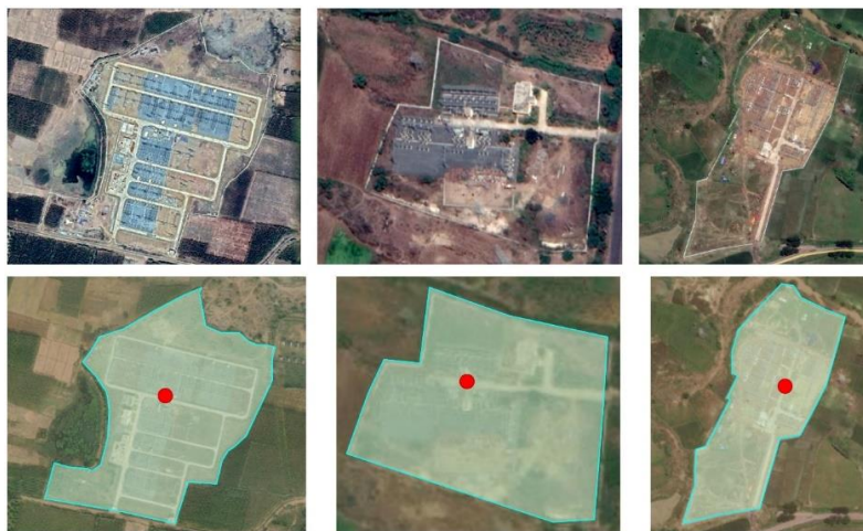
Figure-1. Upper images show samples of few substation showing the boundary, substation infrastructure, internal path and vegetations. Below images show extracted substation boundaries.
